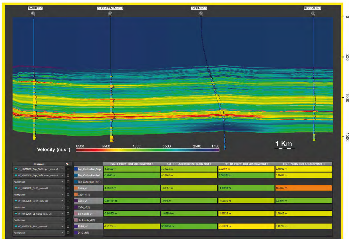
Figure 5-9: Processed velocity model along arbitrary line through the 4 wells in the seismic area and QC control on converted horizons.
